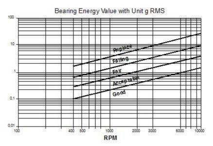
The diagram above is only a guide to interpret the Bearing Energy value. If vibrations of other causes (flow surge, gear mesh) are within in the frequency range 3200-20000 Hz, this can give a high bearing condition value without the bearing being damaged.
